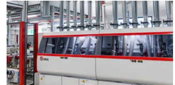
Fully automatic edge coating (glue or zero-joint edge) ▶
