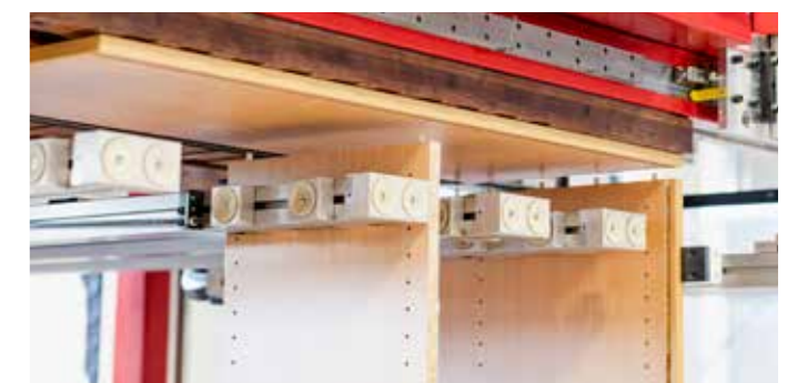
Semi-automated grouting of components in cabinet production ▶
