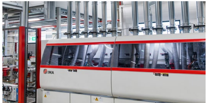
▶ Plant 2 Fully automated edge coating (glue or zero-joint edge)
