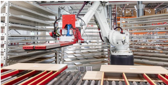
▶ Plant 2 Intermediate storage with robot-controlled sorting
